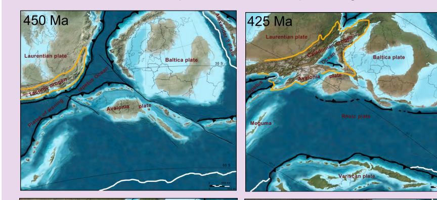
Qualitatively our model attempts to simulate the Larentia Baltica collision by having a trapezium shaped colliding continental block. This creates a collision that propagates along the subduction zone.
