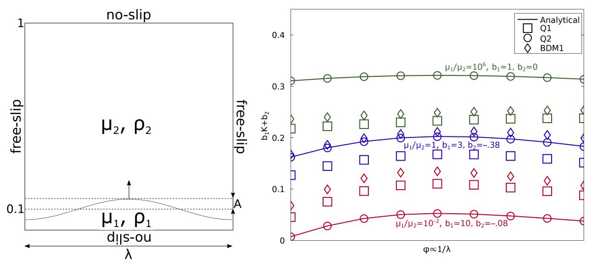
Figure 4: Benchmark setup for Rayleigh-Taylor instability. The jump in density and viscosity is following a small perturbation of amplitude A at z = 0.1. For different viscosity contrasts and wavelengths  $\lambda$  the growth factor K has been computed.  $b_1$ ,  $b_2$  have been chosen such that the plots fit into one figure. such that the plots fit into one figure the plot fit into plot the plot fit plot fit
