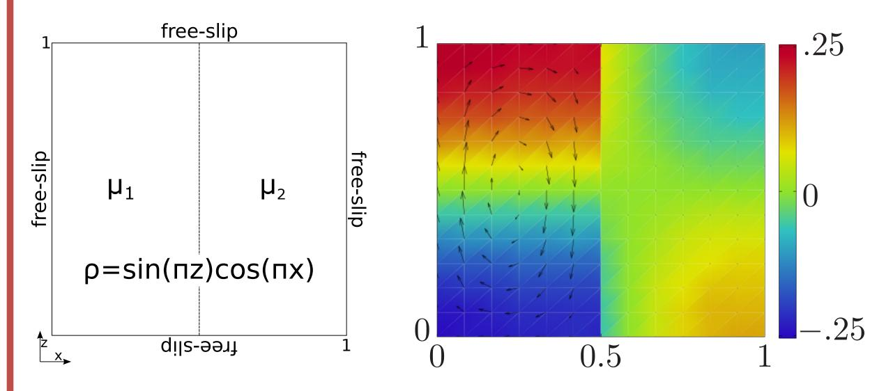
Figure 2: Benchmark setup with lateral viscosity jump. Analytical velocity (arrows) and pressure (colorbar) solution for  $\mu_1 = 1$ ,  $\mu_2 = 10^3$ .
