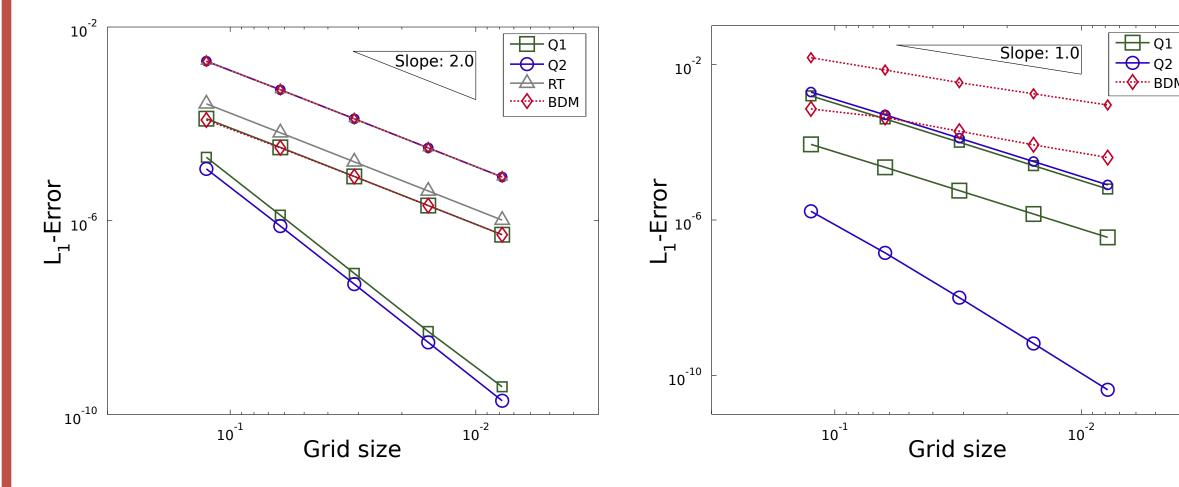
Benchmark with lateral viscosity jump and free-slip boundaries [6],  $\mathbf{f} = (0, \sin(z\pi) \cos(x\pi))^{\mathsf{T}}$ . It has been computed for  $\mu_1 = \mu_2 = 1$ and for  $\mu_1 = 1$ ,  $\mu_2 = 10^3$ , see Fig. 3. As the Raviart-Thomas element does not lead to convergence for discontinuous viscosity, its plot is omitted for the variable viscosity setup.
