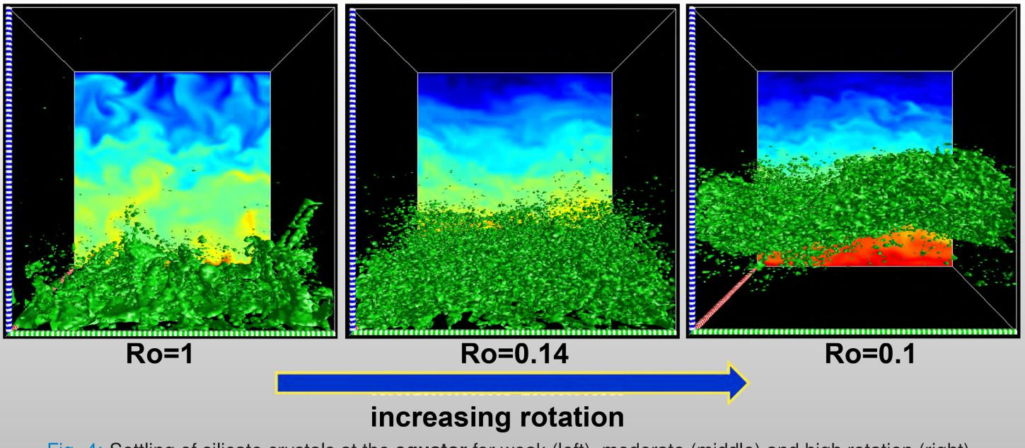
Fig. 4: Settling of silicate crystals at the equator for weak (left), moderate (middle) and high rotation (right).
