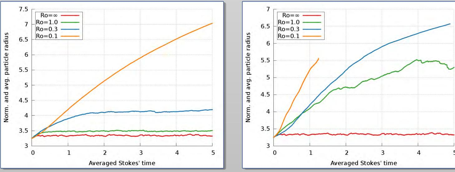
Fig. 7: Evolution of the crystal radius at the **pole** for different rotation rates.
