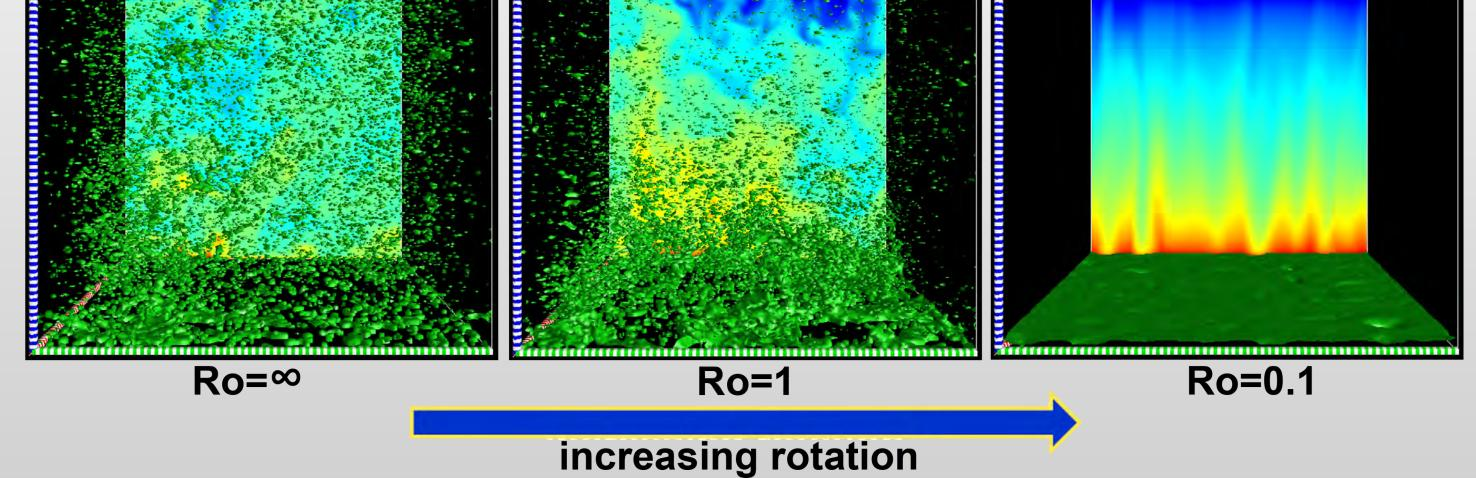
Fig. 3: Settling of silicate crystals at the **pole** without rotation (left), weak rotation (middle) and high rotation (right). In the background the temperature field.
