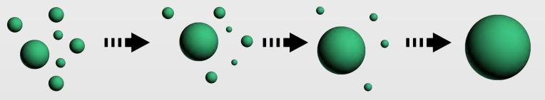
Fig. 6: Principle of Ostwald Ripening: Smaller crystals dissolve, larger crystals grow on behalf of small crystals.
